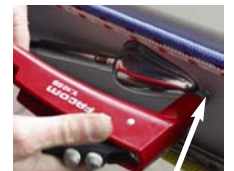
fixing a safety rivet
